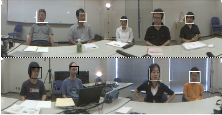
Fig. 4. Typical output from the program showing two 180 degrees sections on top of each other. Detected faces are shown with a white or black square.
