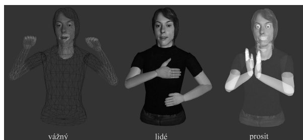
Fig. 5. The animation model for three signs: wire-frame topology, textured and blended rendering
